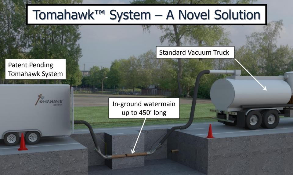
The Tomahawk<sup>™</sup> System restores deteriorated pipes using abrasives and a high-volume, low-pressure airstream to clean and dry the pipe in preparation for lining without using water.
