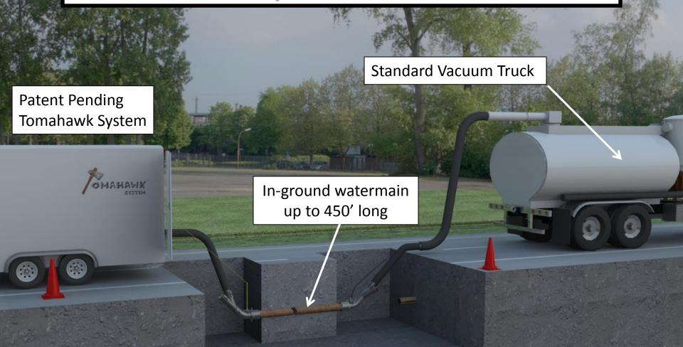
The Tomahawk™ System restores deteriorated pipes using abrasives in a high-volume, low-pressure airstream to clean and dry the pipe in preparation for lining without using water.
