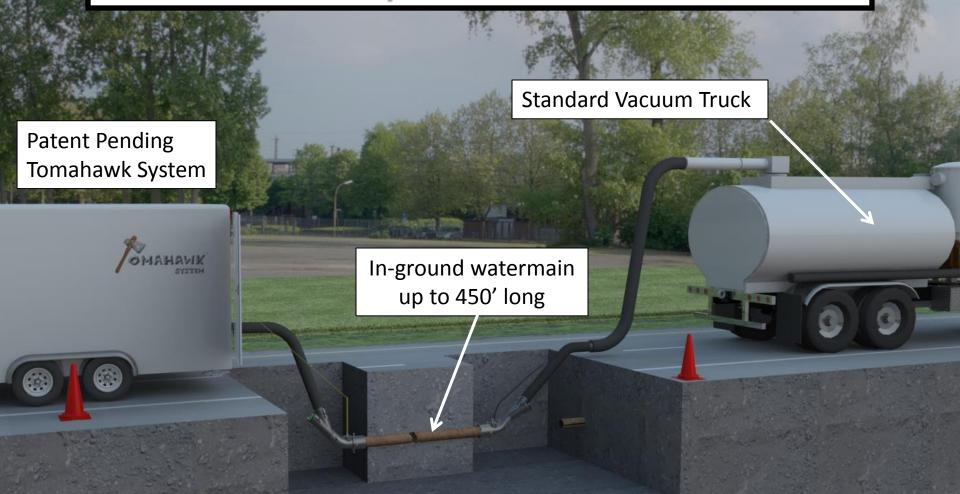
The Tomahawk™ System restores deteriorated pipes using abrasives and a high-volume, low-pressure airstream to clean and dry the pipe in preparation for lining without using water.
