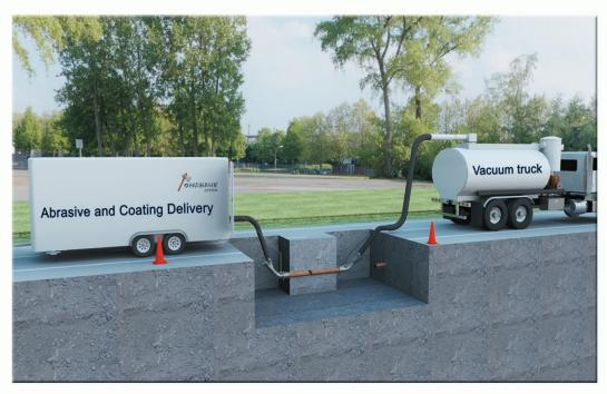
Meets or exceeds cleaning and surface preparation requirements per ASTM F3182-16
