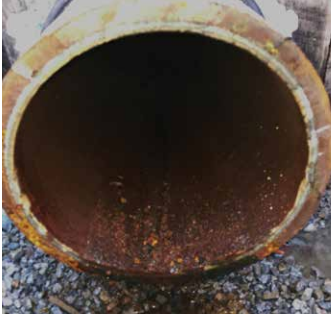
Left photo shows 12-inch CML-lined, corroded cast iron pipe under rail line. Right photo shows a pipe joint and prepared CML coating after removal of corrosion products with airborne stone.
