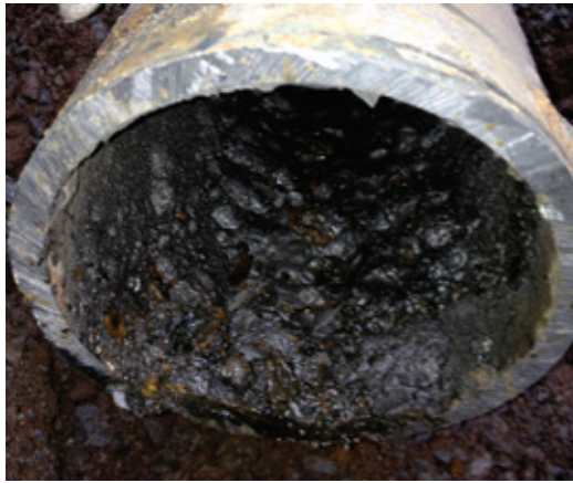
Left and centre: 6-inch, 357 foot CI water main prior to Tomahawk cleaning. Right: same pipe after cleaning.
